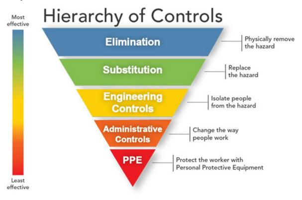
**Elimination** Physically removing hazard is the most effective control. eg employees must work high above the ground, the hazard can be eliminated by moving the piece they are working on to ground level to eliminate the need to work at heights.
